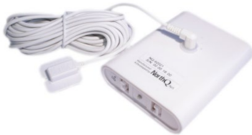
Figure 32 - Z-Wave Data Logger for E-meters ( http://manual.zwave.eu/backend/make.php?lang=en&sku=NOQ_NQ-9021 )
